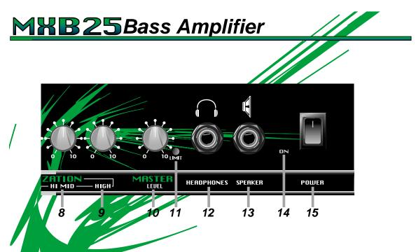
**9: HIGH:** Use this control to adjust the high frequency response of the amplifier. Rotating the control counterclockwise reduces the high frequency output. Rotating the control clockwise increases the high frequency output. The High control provides a range of 33dB of boost or cut at 10kHz.
